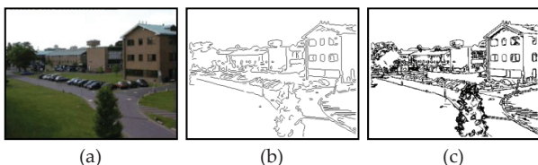
Figure 1. Edges have changes in shape and position. (a) A sample scene with waving trees, and (b) its extracted edges. (c) The accumulation of 100 edge frames shows the variation of the edge's movement. In (c), the building's edges are thin, which depict small movement, while the trees' thick edges justify high movement variations.
