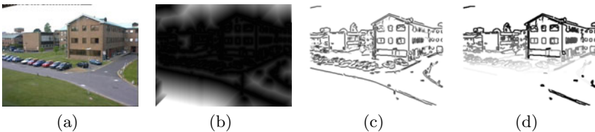
Fig. 3. Distance Map used in Hossain et al. method and the proposed method. (a) A sample reference frame. (b) CDM made from 50 training frames. (c) SDM made from 50 training frames. (d) Edge segment labeling map over the SDM.
